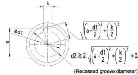
Set the diameter of the recessed groove (d2) so that it is larger than the corner of the keyway
