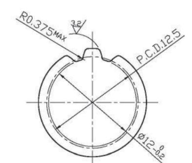
Detailed drawing of spline section
