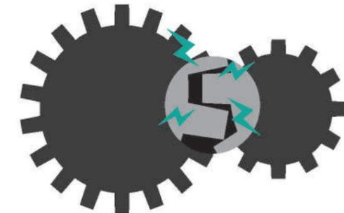
▲ The unsmooth torque transmission caused by the abrasion or interference of gear in conventional mechanism.
