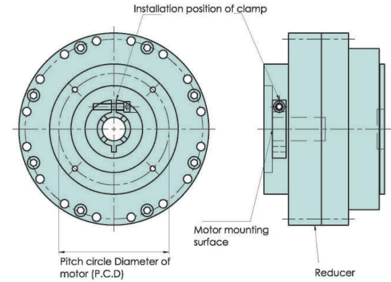
1. Place motor shaft key and reducer input shaft key way in a straight line, and insert motor shaft into reducer input shaft.
