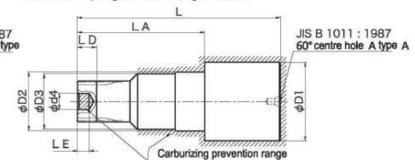
Note: The above drawing shows the shape before the additional machining is performed. Check the dimensions of each section.
