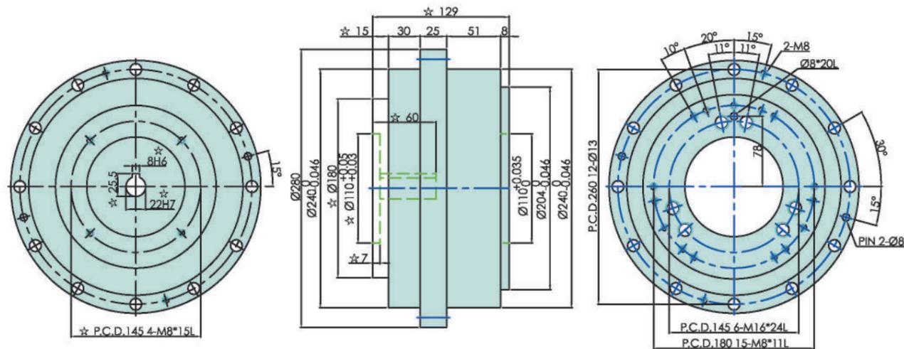
1. "☆"The dimensions modify with motor specification.
