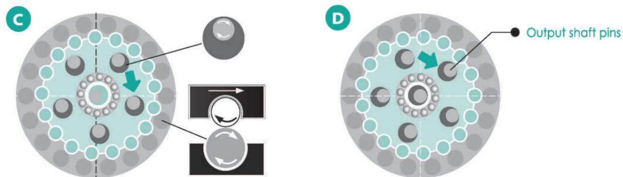
6.While internal rollers turning counter-clockwise accompanied with roller disc, this make rotation of internal rollers and external rollers separately follow individual center axis due to mesh transmission.
