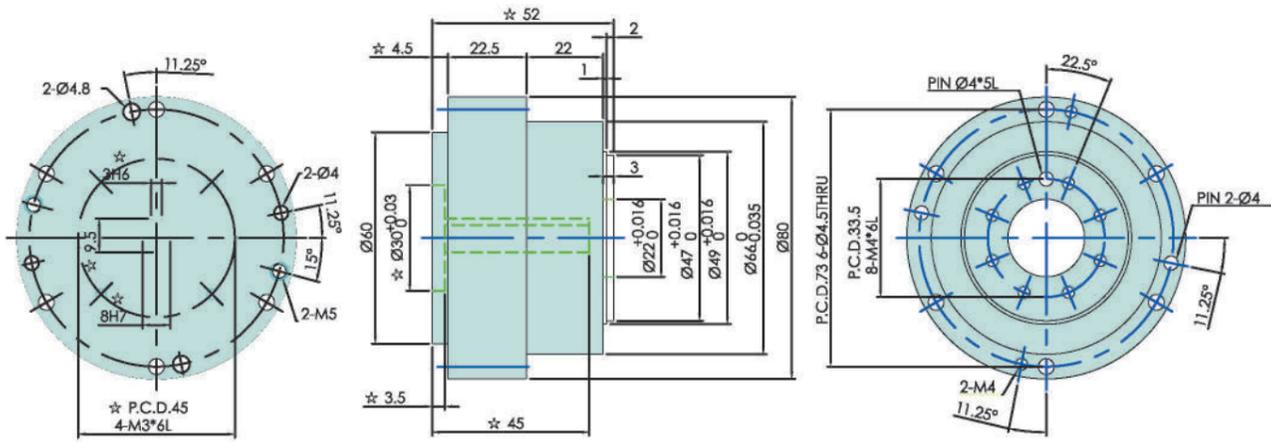
1. "☆"The dimensions modify with motor specification.
