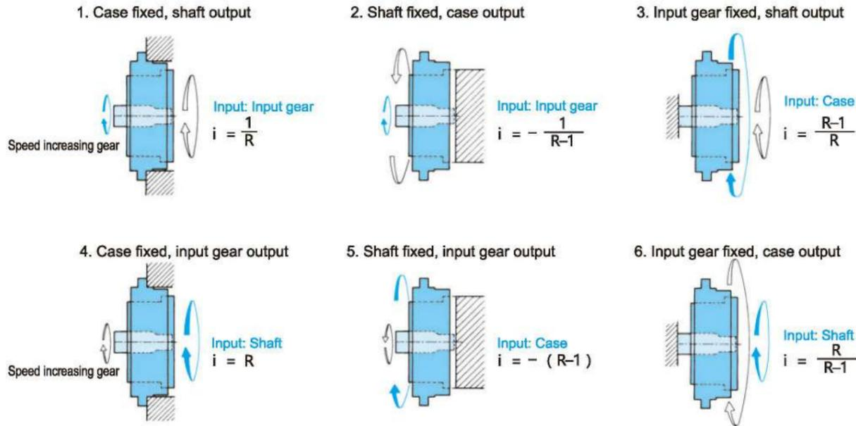
•The "i" in the above equations signifies the speed ratio of the output for the input in each case. The "+" signifies the output in the same direction as the input and the "-" signifies the output in the opposite direction to the input.
