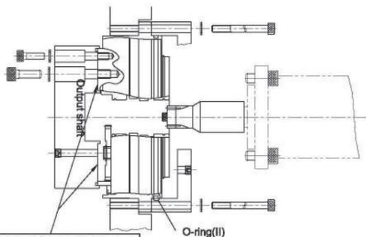
Use fluid sealant for mounting surface
