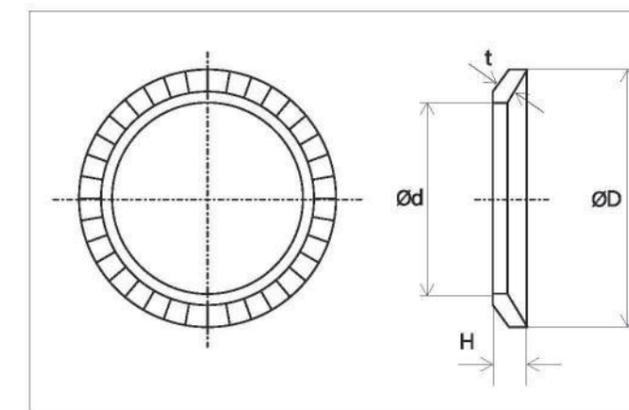
Note: When using any equivalent washer, select it with special care given to its outside diameter.
