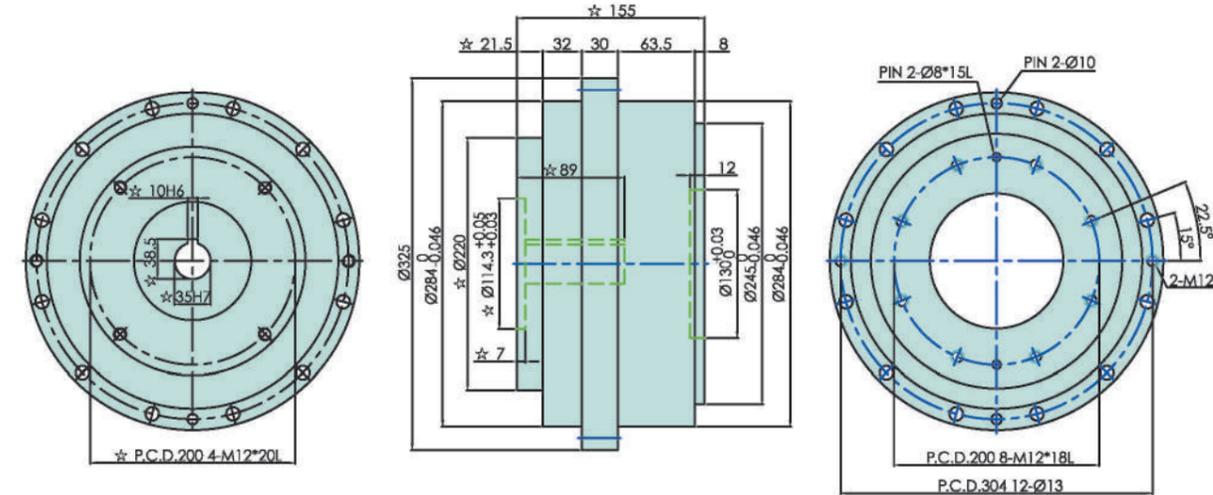
1. "☆"The dimensions modify with motor specification.
