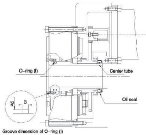
Dimensions for O-ring (I) seal(for reference) (Unit: mm)
