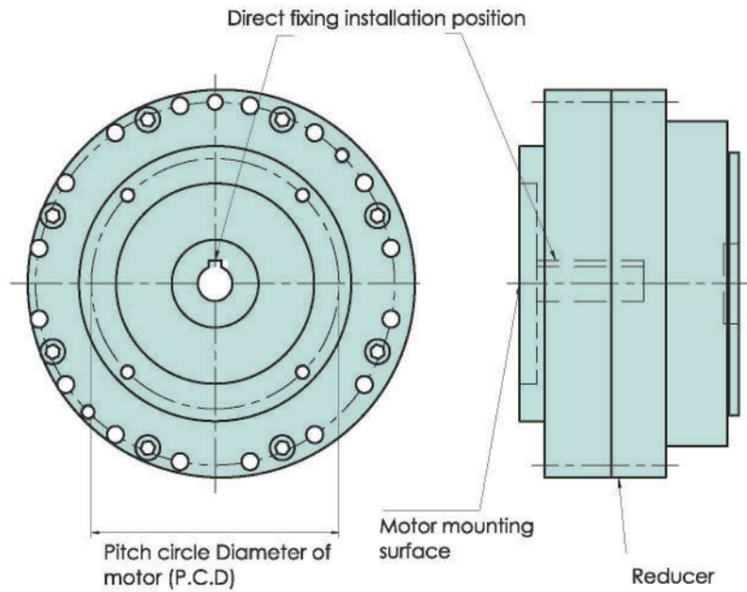
1. Place motor shaft key and reducer input shaft key way in a straight line, and insert motor shaft into reducer input shaft.
