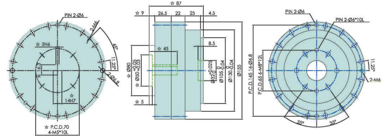
1. "☆"The dimensions modify with motor specification.
