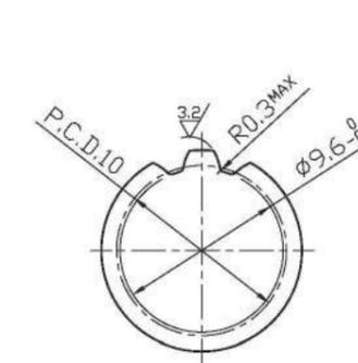
Detailed drawing of spline section
