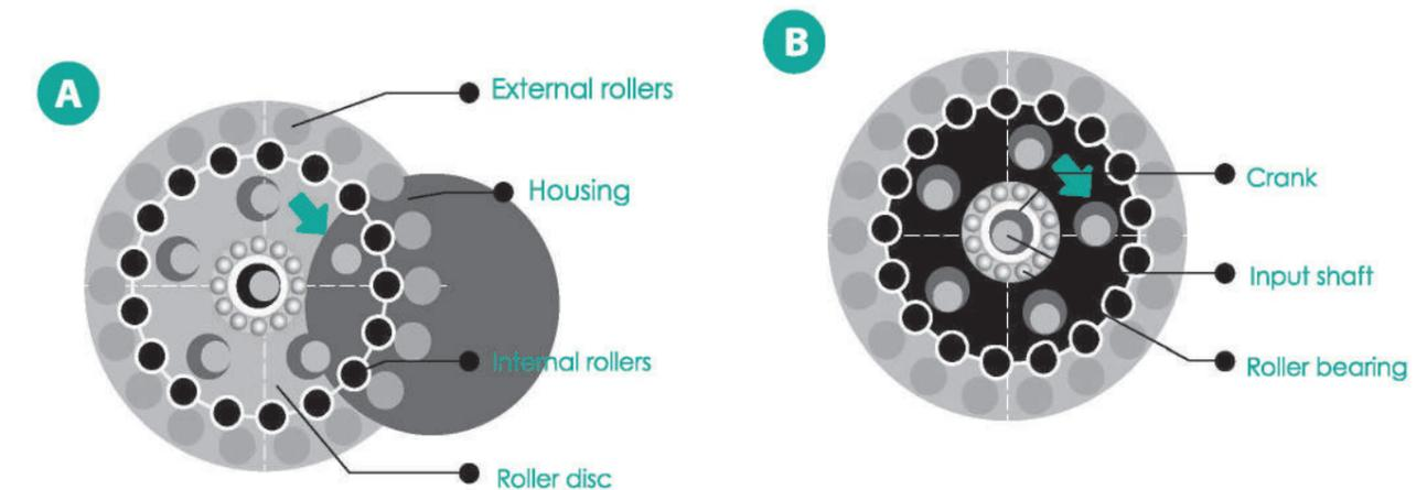
1. Cylindrical external rollers mounted in robust housing.
