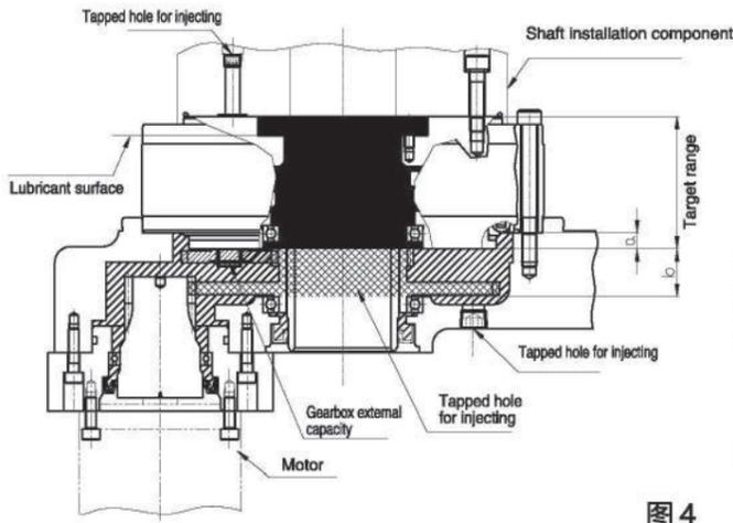
Vertical shaft installation (with shaft facing downward)
