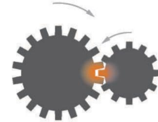
▲ Conventional spur or helical gear must bear over-load impact due to merely one-tooth engagement in each mesh.
