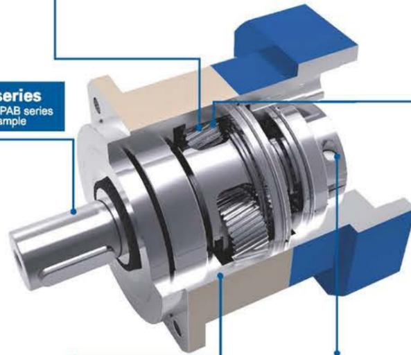
The output planet carrier adopts integral (double support) structure design. The large span of the front and rear bearings is distributed inside the box body, forming a stable integrated structure to ensure high torsion rigidity and accuracy.
